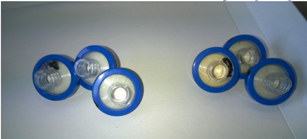
Figure 9: The Convergence MFI/SDI 0.45-micron filters used to derive the MFI/SDI of the ASRO feed water (left) and the BWRO feed water (right) (date: June 19, 2015).
