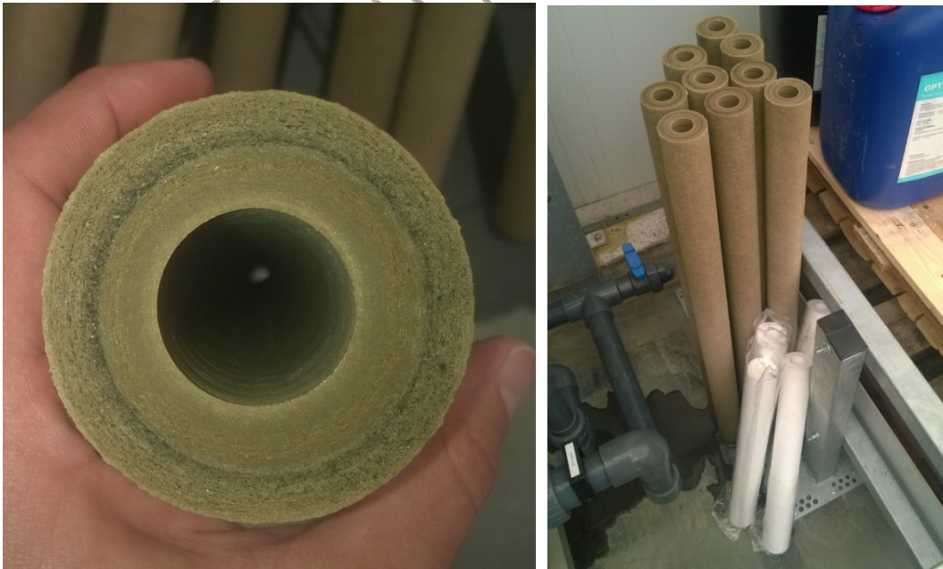
Figure 9: The Convergence MFI/SDI 0.45-micron filters used to derive the MFI/SDI of the ASRO feed water (left) and the BWRO feed water (right) (date: June 19, 2015).
